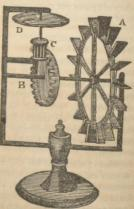
trundles placed on its opposite sides; and on the top of each axis of the trundles, may be a round plate, representing a mill-stone: so that this model has all
